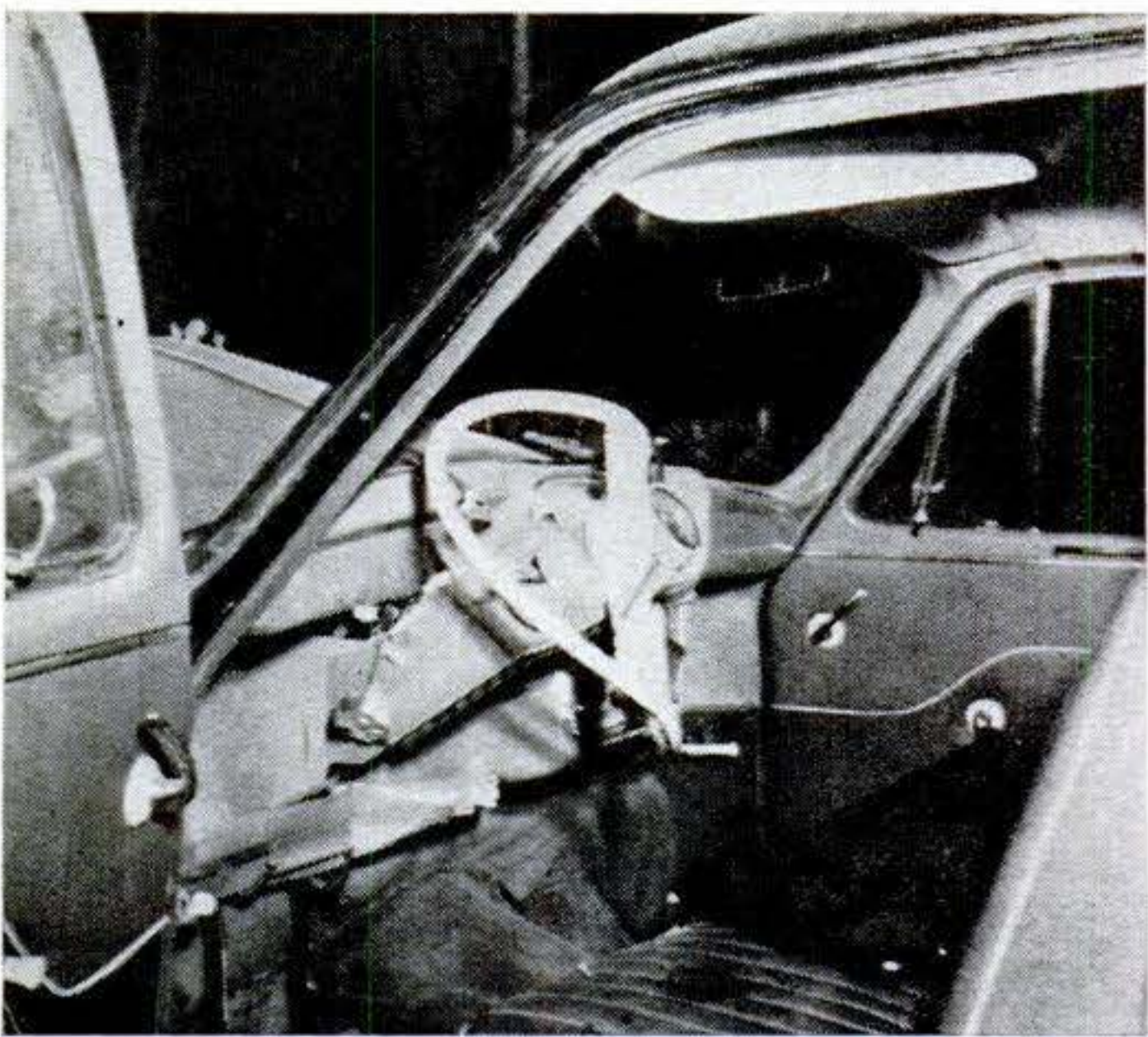
WINDSHIELD POPPED OUT WHOLE in the Hillman-vs.-tree accident, protecting driver and passenger. They were injured, but not seriously.
